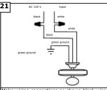
Make wiring connections as shown black wire from house to black wire from fan. White wire from house to white wire from fan. Connect all green ground wires to ground wire from house. Refer to diagram above.
